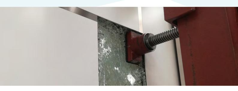
The company VEYNA, in collaboration with his partners, have succeeded all the test for security doors RC2 with security glass of class P4. All our panels are gived gratis to pass the tests in the research entities or other control bodies. Security doors RC2 or RC3 enrich our offer and give possibility to buy more solid doors in the producers. They still gard their news and interesting designs. The tests were done for doors in alu.
